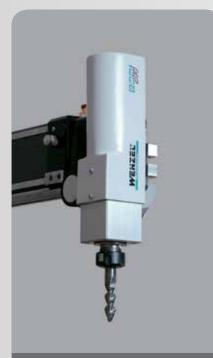
Milling and drilling head DMH 200 For milling in soft materials (foam, clay, ...) spindle capacity 200 watt, max. speed 7000 rpm, convertible to CMM universal mounting head.
