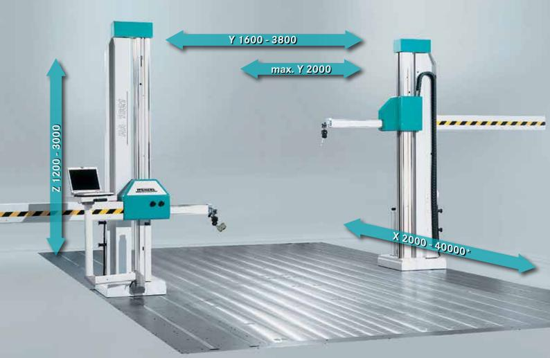
\* All machines are available as standard up to X = 40.000 mm, 500 mm increments, larger X- and variable Y- and Z-ranges on request. For technical information, please refer to the respective data sheet.
