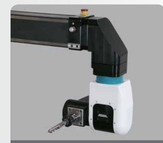
Additional emergency stop on the milling head (Excalibur)
