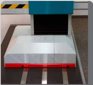
**Switching boards for RA and RAplus** Additional collision protection in the X-axis on RA and RAplus machines.
